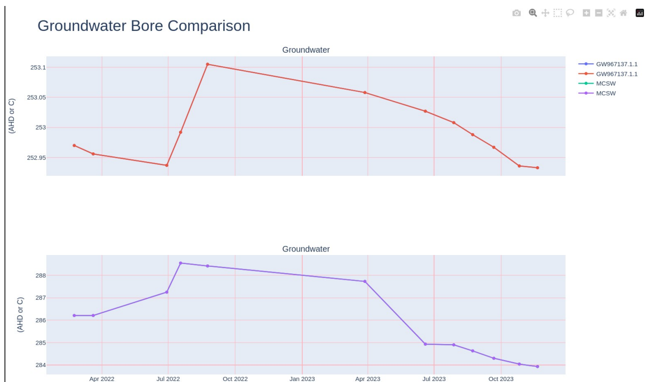
Fig2: Elfin Crossing GW967137.1.1 (top in red) has only fallen 17 centimetres compared to nearly 4 meters at Middle Creek South Well (bottom in blue) since it peaked on July 18 2022. Note that the differences in scale on the y axis
