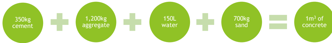
Figure 1: Ingredients in a typical concrete mix
