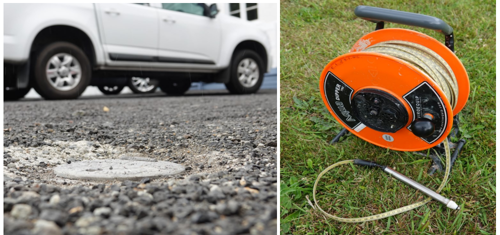
Above left: The flush cap of a piezometer hole in the carpark at St John's Anglican Church at the top of Seddon Street.
