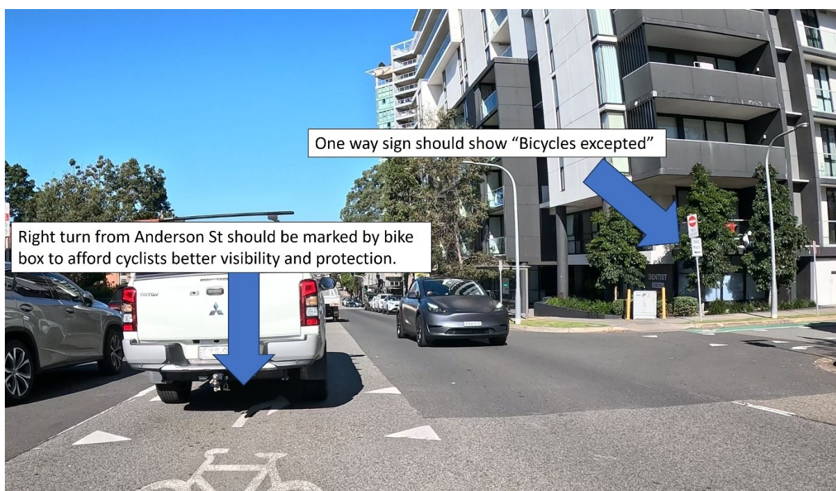
Figure 9 A marked on road bike box from Anderson St to McIntosh St would be modern convention, affording better protection for cyclists. The "No Entry" sign opposite should indicate "Bicycles excepted"
