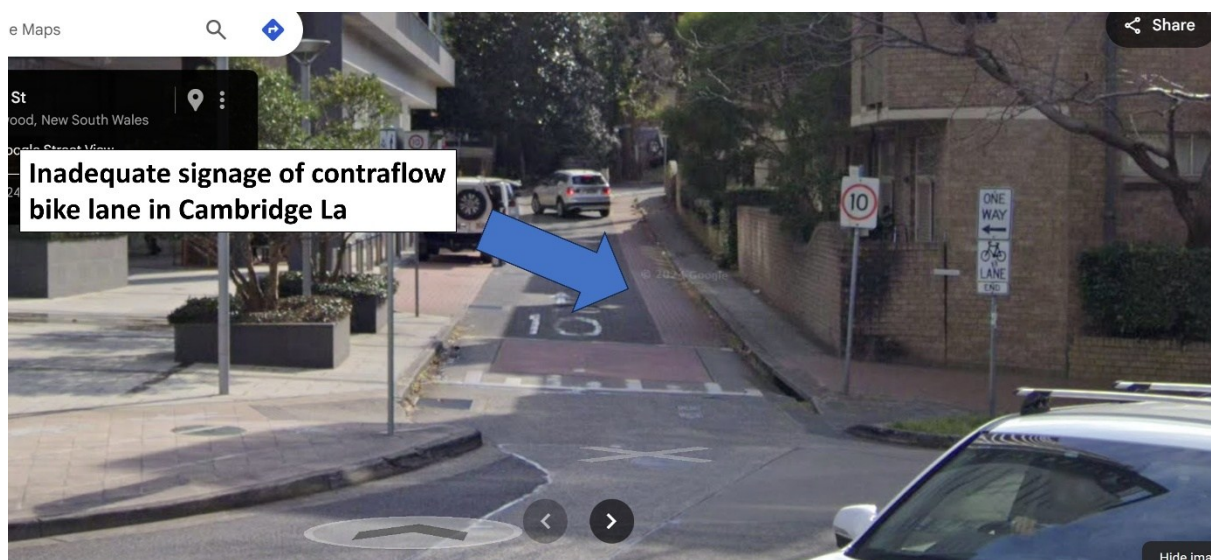
Figure 4 Inadequate signage of contra-flow lane in Cambridge Lane
