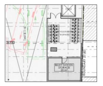
Fire separation for consideration by the certifier – wall between bulk goods storage and the substation. The bulky goods storage (depending on management of access) may contain hazardous goods such as a portable BBQ.
