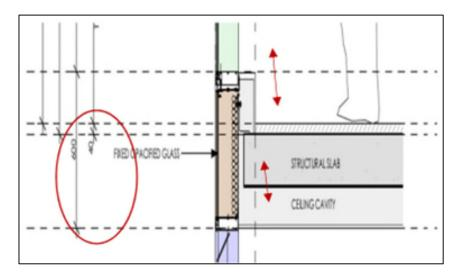
The transome is 1000mm, and fixed vision glass is 800mm. Subtracting the fixed vision glass from transom leaves 200mm. 200mm of opacified glass, fixings and 40mm of flooring meant that the curtain wall construction has vertical protection (assumed) to 240mm.
