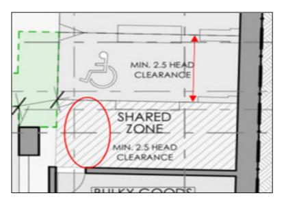
On drawing SK10 P24, there appears to be a substation pit above the accessible parking space. Recommendation for services designer/engineer to consider relocation of this pit. Otherwise, the construction of this space must be in accordance with AS2890.6-2022 – car parking spaces for disabilities
