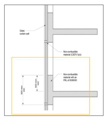
Separation of external window openings to prevent spread of fire between levels must cover 900mm, with 600mm at minimum from the edge of floor above. Red arrows are critical information gaps where it is unknown how this curtain wall design will achieve compliance, or a performance solution warranted for the proposal.
