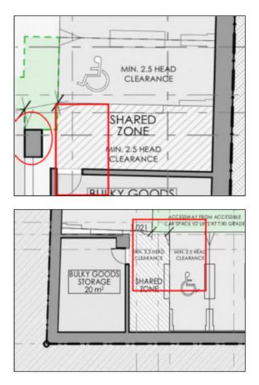
In the above screenshot (western end of basement), there is only 1.021m of clearance between the edge of accessible parking space and the edge of adjoining parking space. The length of space and parking angle meant that a big utility vehicle, as is now common in Australia, will not only reduce the 1.02m clearance, and make it difficult to exit shared zone if there is concurrent access to bulky goods storage.
