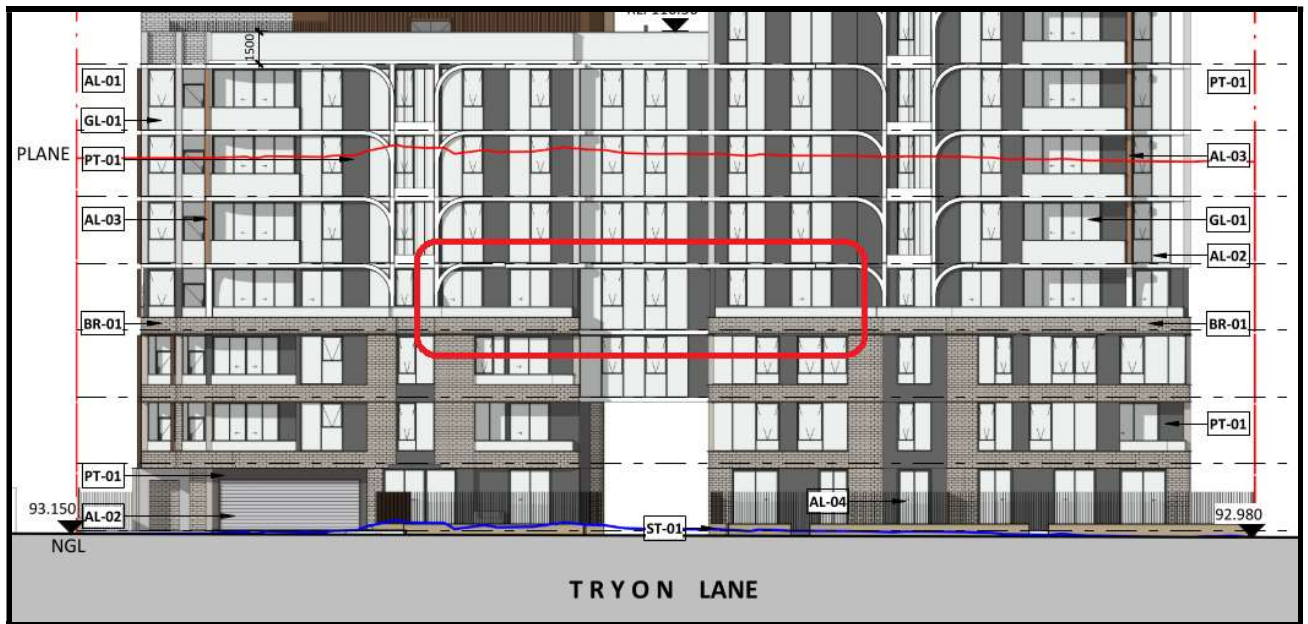
Figure 5 inadequate privacy measures between adjoining balconies of Buildings C and D (elevation view)
