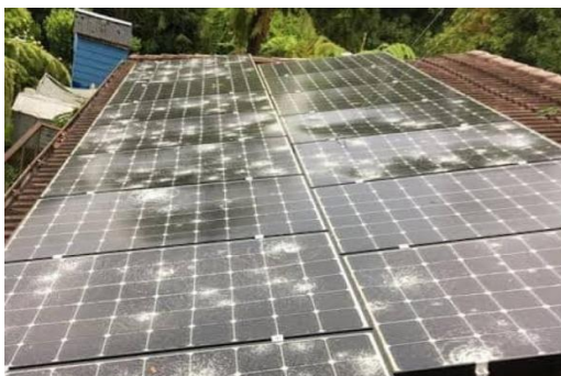
Solar panels damaged by hail. Off to landfill!
