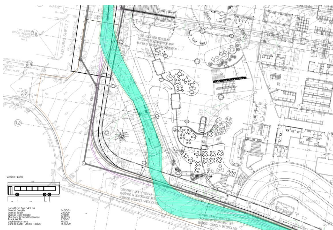
Figure 27 - Swept Path of a Typical 14.5m Coach Bus through the Porte Cochere
