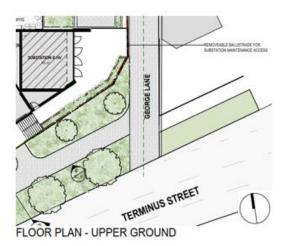
Any required distribution substation will need to be located within the property (in a suitable and accessible location) and be protected (including any associated cabling not located within a public road / reserve) with an appropriate form of property tenure as detailed in the attached copy of Endeavour Energy's 'Land Interest Guidelines for Network Connection'.
