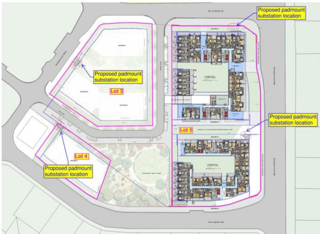
Figure 8: Proposed Endeavour Energy substation Infrastructure
