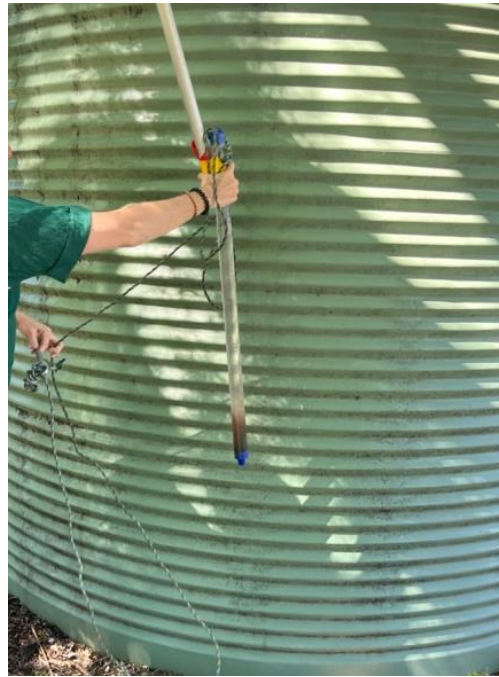
Measuring a domestic tank approximately 6-8 years old. Never cleaned. Positioned under a tree canopy and has sieve on the inlet
