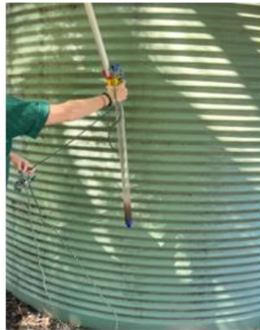
Measuring a domestic tank approximately 6-8 years old. Never cleaned. Positioned under a tree canopy and has sieve on the inlet
