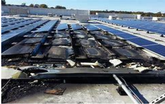
Remains of a solar panels fire
