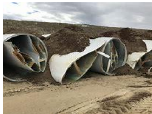
Disposing of cut up wind turbine blades
