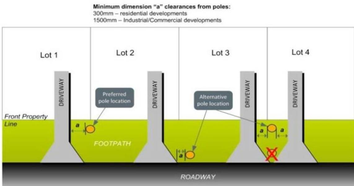
The minimum separation to the skirting of the proposed driveway is regarded as the minimum that would be acceptable / safe for anyone properly using the driveway (and for which depending on the circumstances appropriate protective devices may be required) and failing the foregoing an asset relocation may be required.
