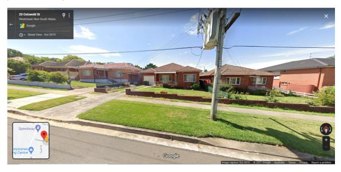
Driveways need to be appropriately located in relation to poles. Poles with transformers (pole mounted substations) may have an additional earth mat surrounding the pole and should be provided with greater separation to driveways. Repairs and maintenance to poles can occur over extended periods of time blocking driveway access. Source: Google Maps Street View.
