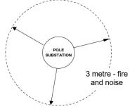
Figure 13 – Fire and noise separation
