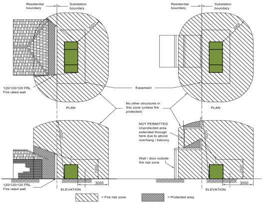
Figure 47 - Typical effect of screen walls
