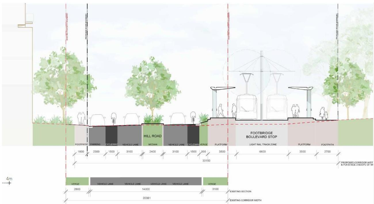
Figure 3: Cross section of Hill Road in Wentworth Point showing existing and proposed allocation of road space (Source: TfNSW / ASPECT Studios)
