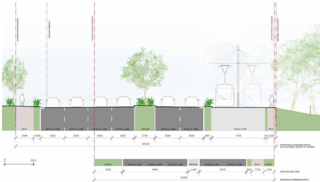
Figure 5: Cross section of Hill Road near Holker Street in Wentworth Point showing existing and proposed allocation of space (Source: TfNSW / ASPECT Studios)
