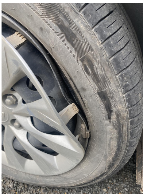
Figure 62 Example of damage to wheel rim from local roads – Goulburn Road (MR79) 52
