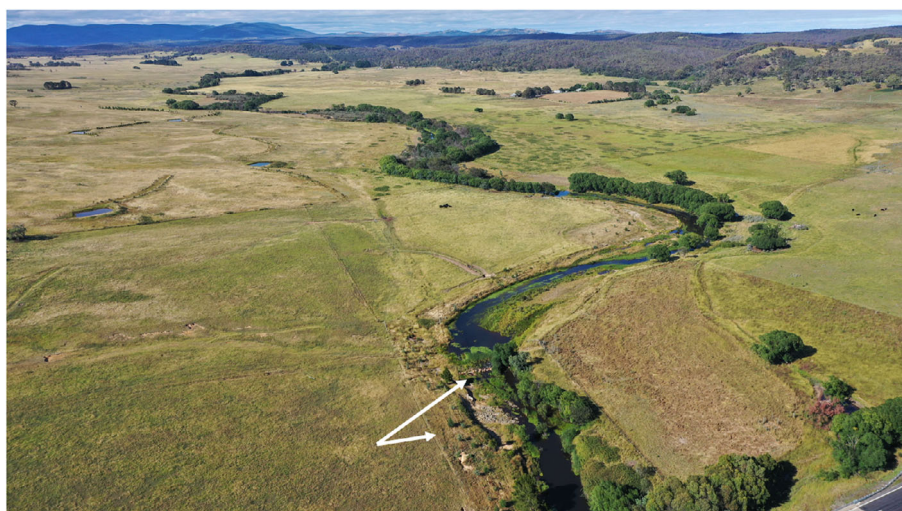
Figure 1. The Mulloon Rehydration Initiative is restoring hydrological function along all degraded reaches of the Mulloon Creek integrated with a research and monitoring program. Seen here in the lower front is a typical 'leaky weir' (long arrow) and fenced riparian revegetation (short arrow).
