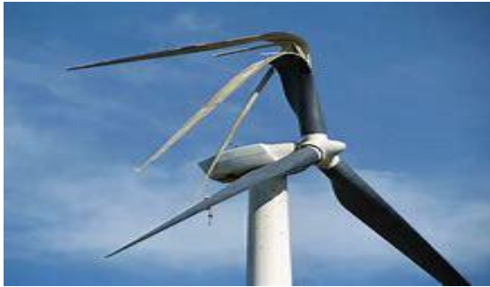
Lightning strike shuts down wind turbine
