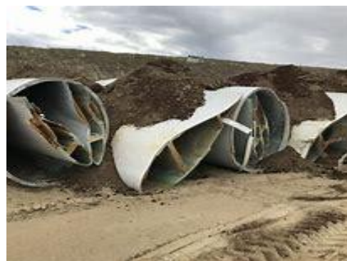
Disposing of cut up wind turbine blades
