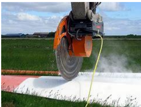
Cutting up end-of-life wind turbine blades
