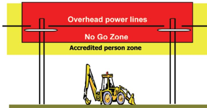
Mobile plant including cranes, excavators, EWPs, earth moving machinery, tipper trucks and concrete placing booms whose design envelope is within the approach distances specified in Table 1 must be controlled by safe systems of work as described in this chapter.
