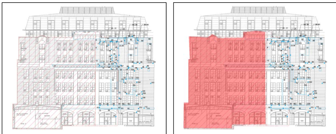
East Elevation showing demolition works in red hatching (left) and highlighted by National Trust for clarity (right). (Source: Heritage Conservation Schedule, Apex Diagnostics, p.280)
