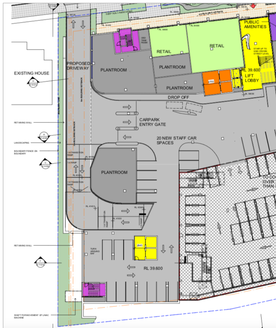
Figure 2: Lower Ground floor plan extract identifying inadequate spatial separation to the western allotments
