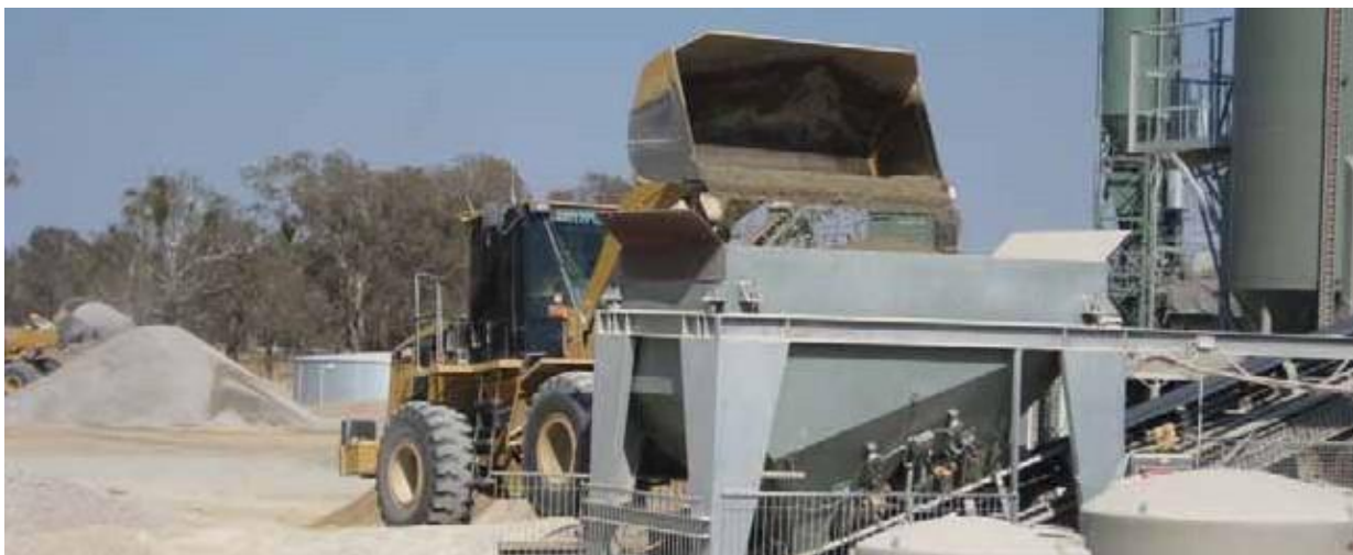
A loader fitted with a broadband reversing alarm rather than a beeper alarm (Abigroup Contractors Pty Ltd)
