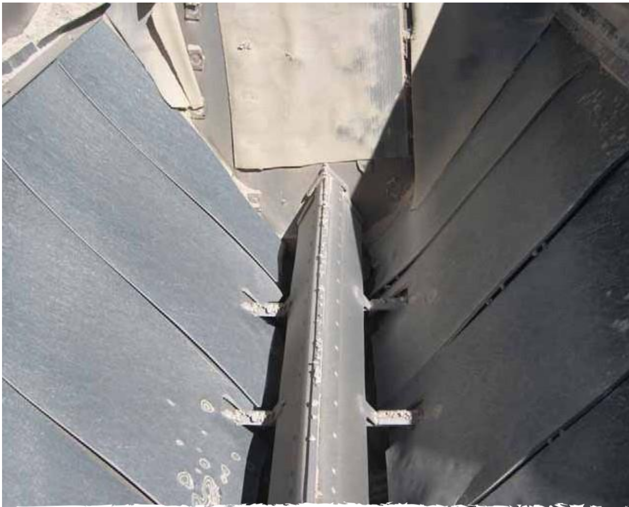
Reduce noise from chutes and bins by lining with damping material (Abigroup Contractors Pty Ltd)
