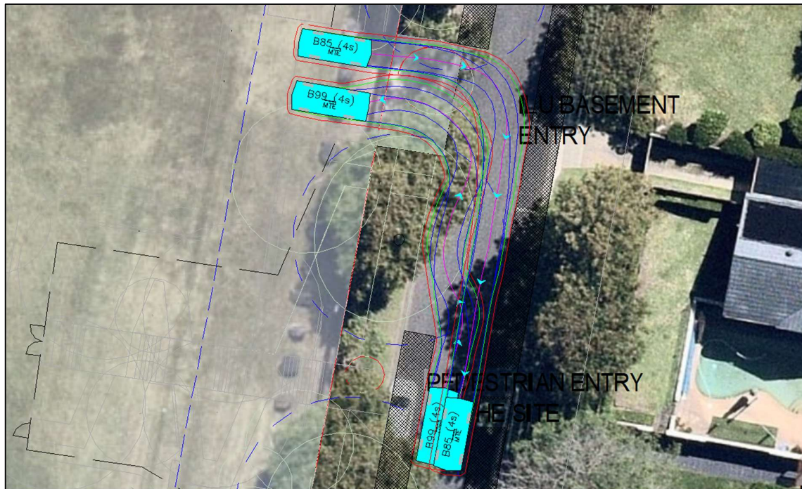
FIGURE 6: B85 PASSING B99 AT COLLEGE CRESCENT NORTHERN DRIVEWAY
