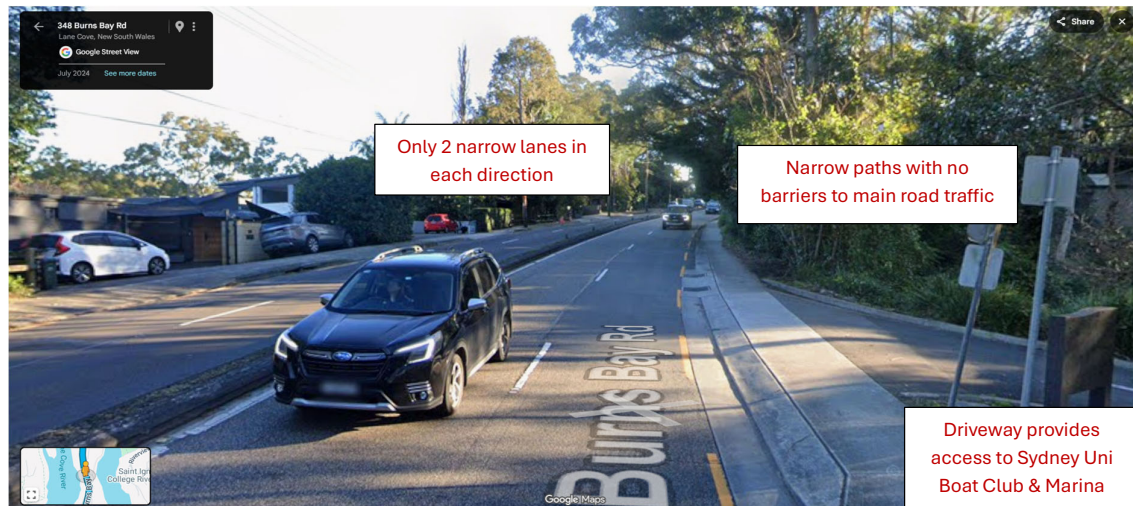
Figure 2: Narrow lanes and pedestrian paths with no barriers to main road traffic
