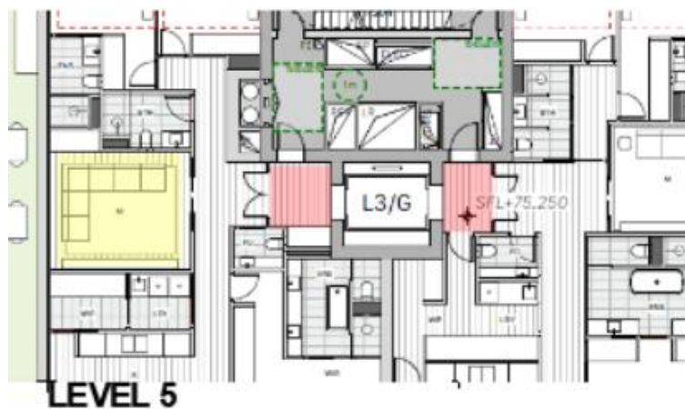
Extract of floor plans with mark-up to highlight circulation issues (Source: Drawings 2102, 2105, and 2107, FJC Studio)
