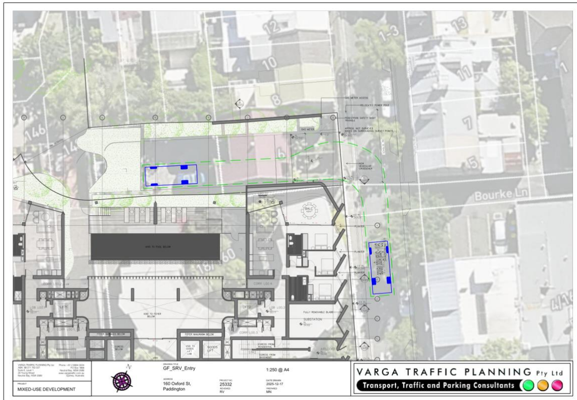
Figure GF_SRV_Entry (Source: Varga Traffic Planning, Transport and Accessibility Impact Assessment, November 2025): Swept path diagram showing the waste collection vehicle (SRV mini rear loader) reversing across Shadforth Street into the basement loading dock. The new vehicular crossover is marked, as are the terrace houses at 5, 7, 9 and 11 Shadforth Street directly opposite.
