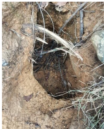
Photo 17 & 18: Site 6 Subsidence Crack 600mm x 300mm – June 2024
