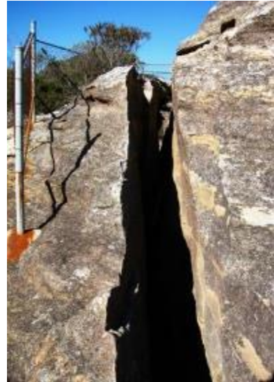
Photos 13, 14, 15 - Mine subsidence cracks – Hassans Walls Reserve – May 2009
