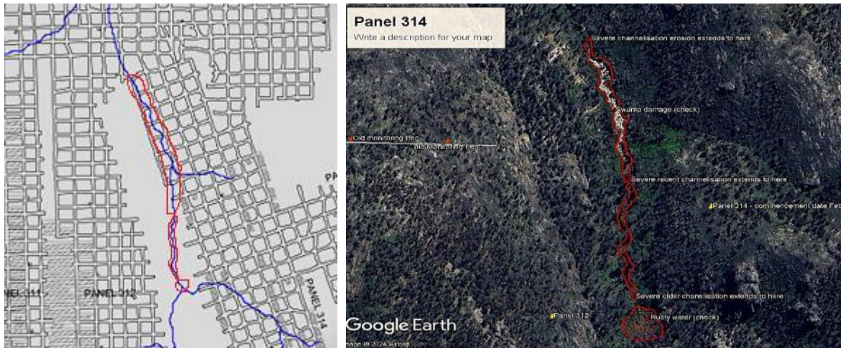
Photo: 76 & 77 Clarence Colliery Panel 314 – Severe channelisation, erosion & dried-up creek in former THPSS
