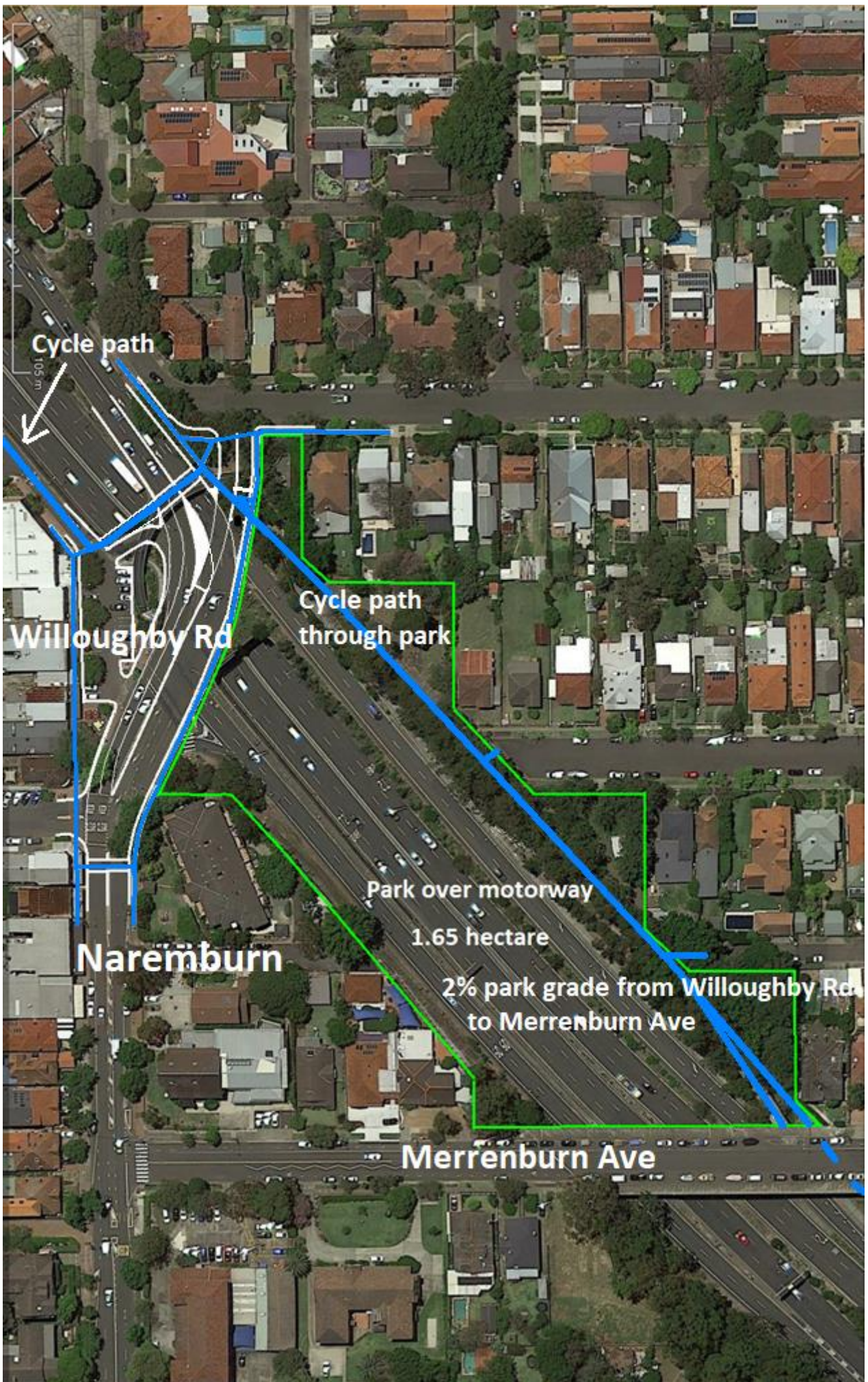
Figure 10.2 – Building a park over the motorway at Naremburn
