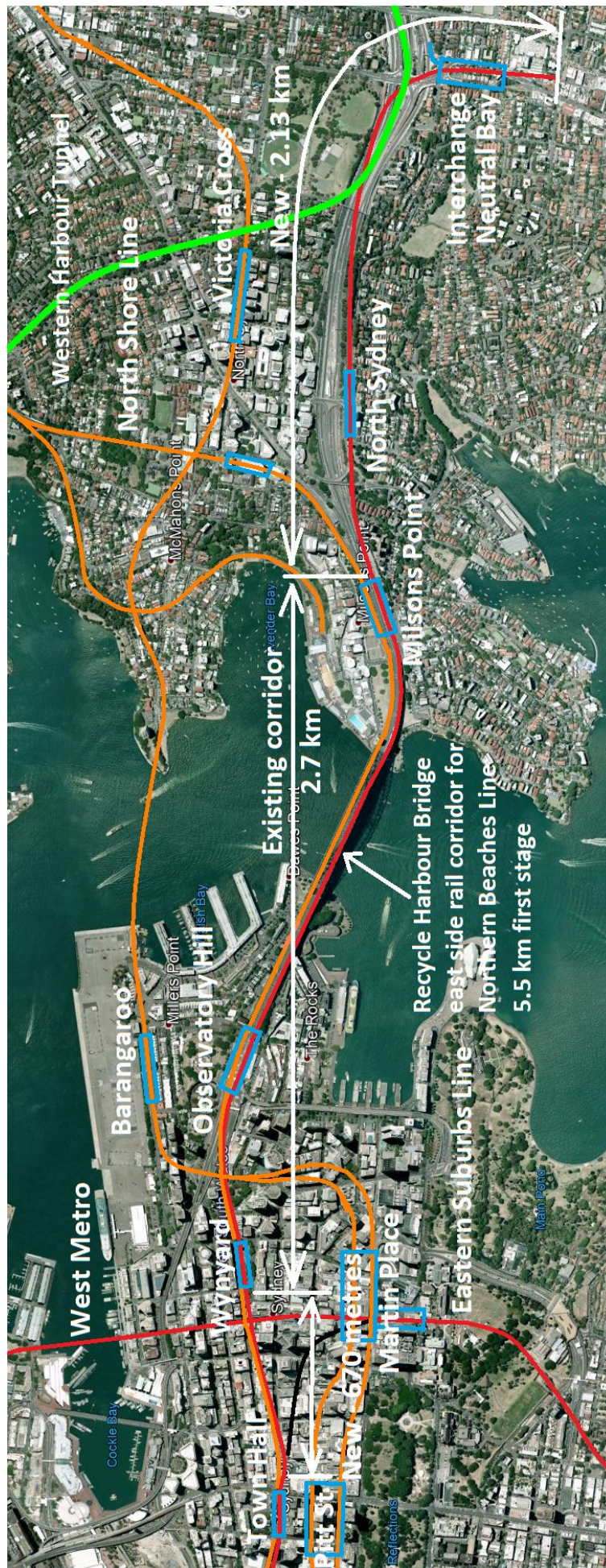
Figure 8.4 – six-lane WHT permits rededication to rail of the former Harbour Bridge rail (tram) corridor from Wynyard to Milsons Point with an underground extension to Neutral Bay
