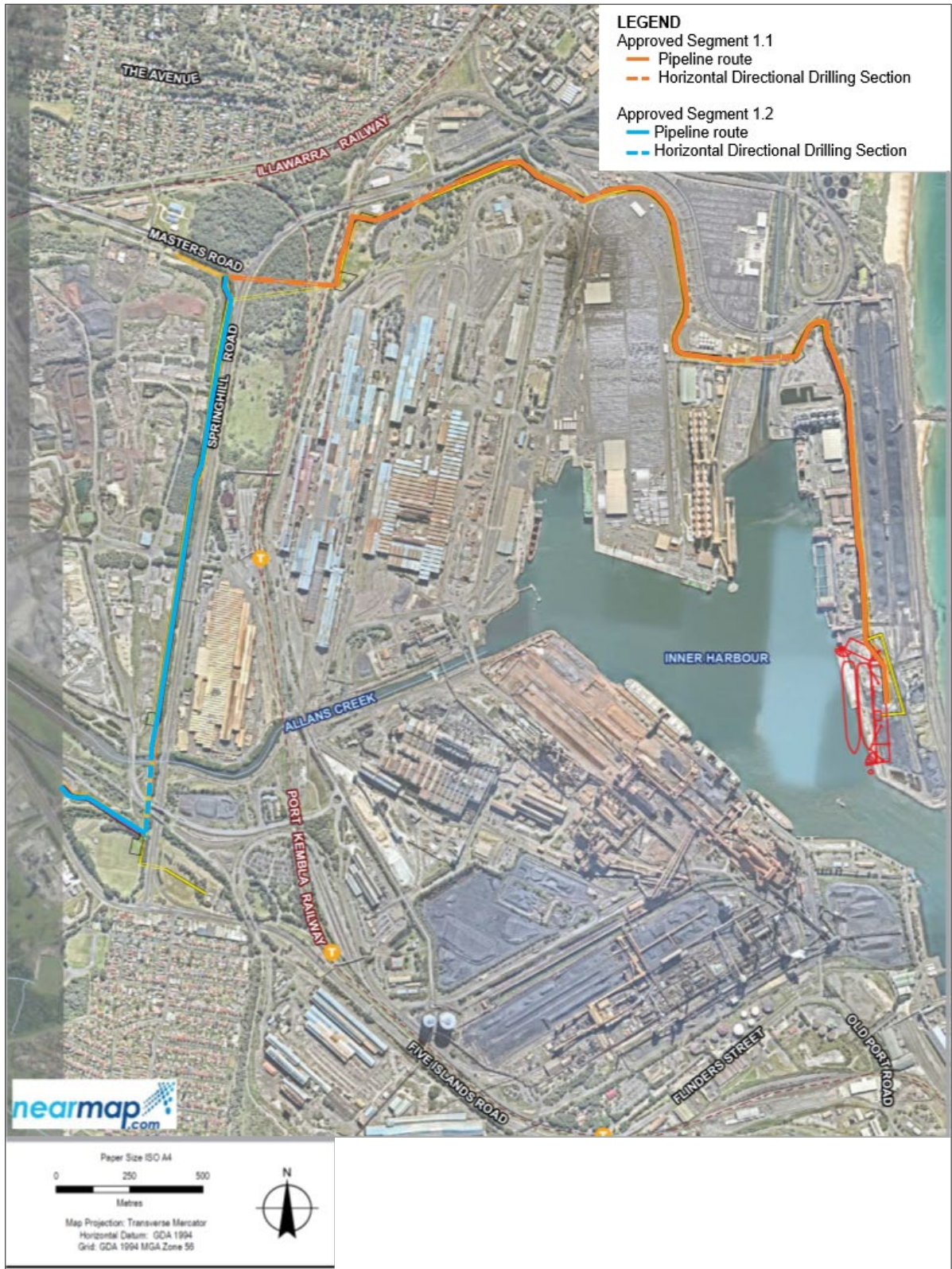
Figure 1 | Pipeline alignment approved under SSI 9471 (Source: Modified from GHD (2018) Port Kembla Gas Terminal Response to Submissions Report)
