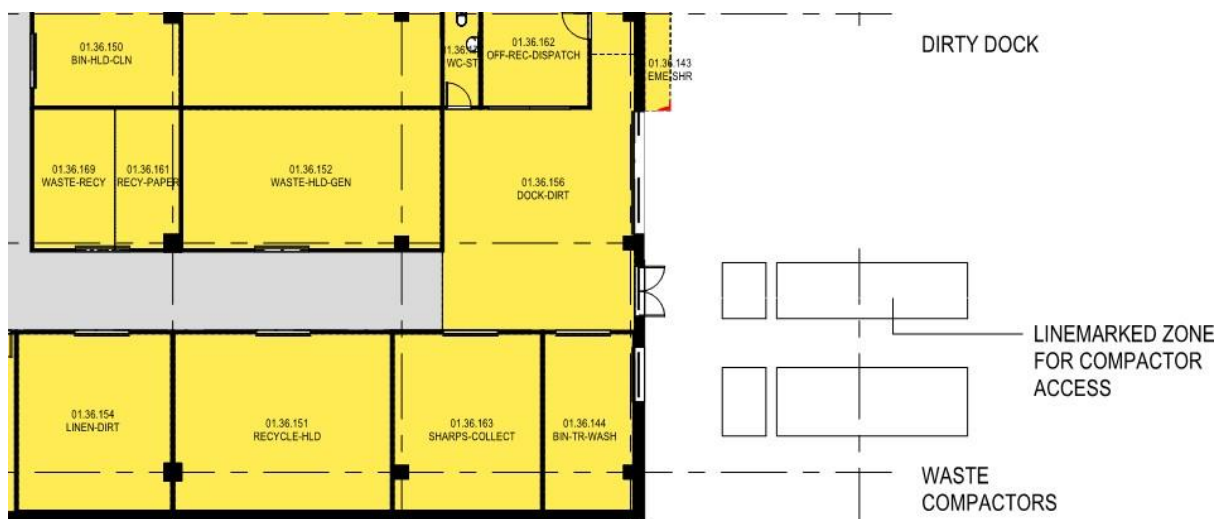
Figure 1: Loading Dock Waste Management Area
