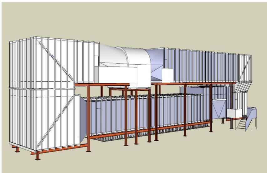
Figure 3: Schematic of the closed-circuit wind tunnel.
