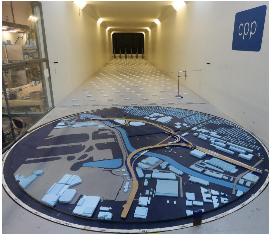
Figure 6: Sydney Airport model including the proposed Sydney Gateway in the wind tunnel.
