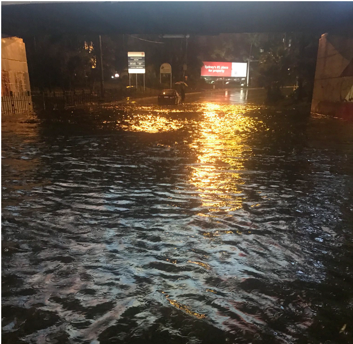
Plate 1: Photo taken during storm of 7 September 2018 showing flooding to the low point in the Robey Street Underpass. The water level against the fence that is located to the left of the road indicates that the depth of inundation was likely to have been in the order of 0.2 to 0.3 metres. [Source: Sydney Morning Herald website]
