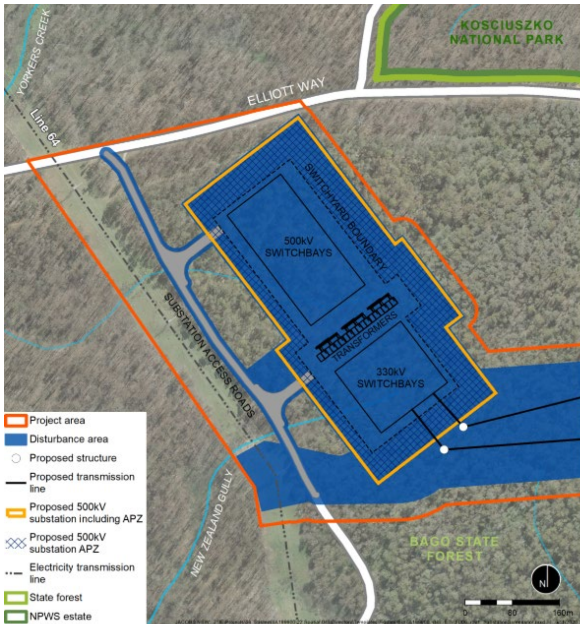
Figure 5-1 Indicative substation layout
