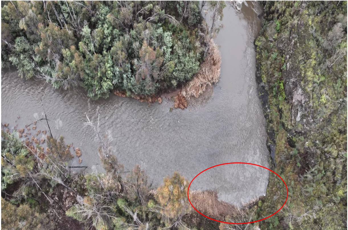
Figure 4: Sediment laden water observed downstream of F10.5 basin on 20/07/2024.
