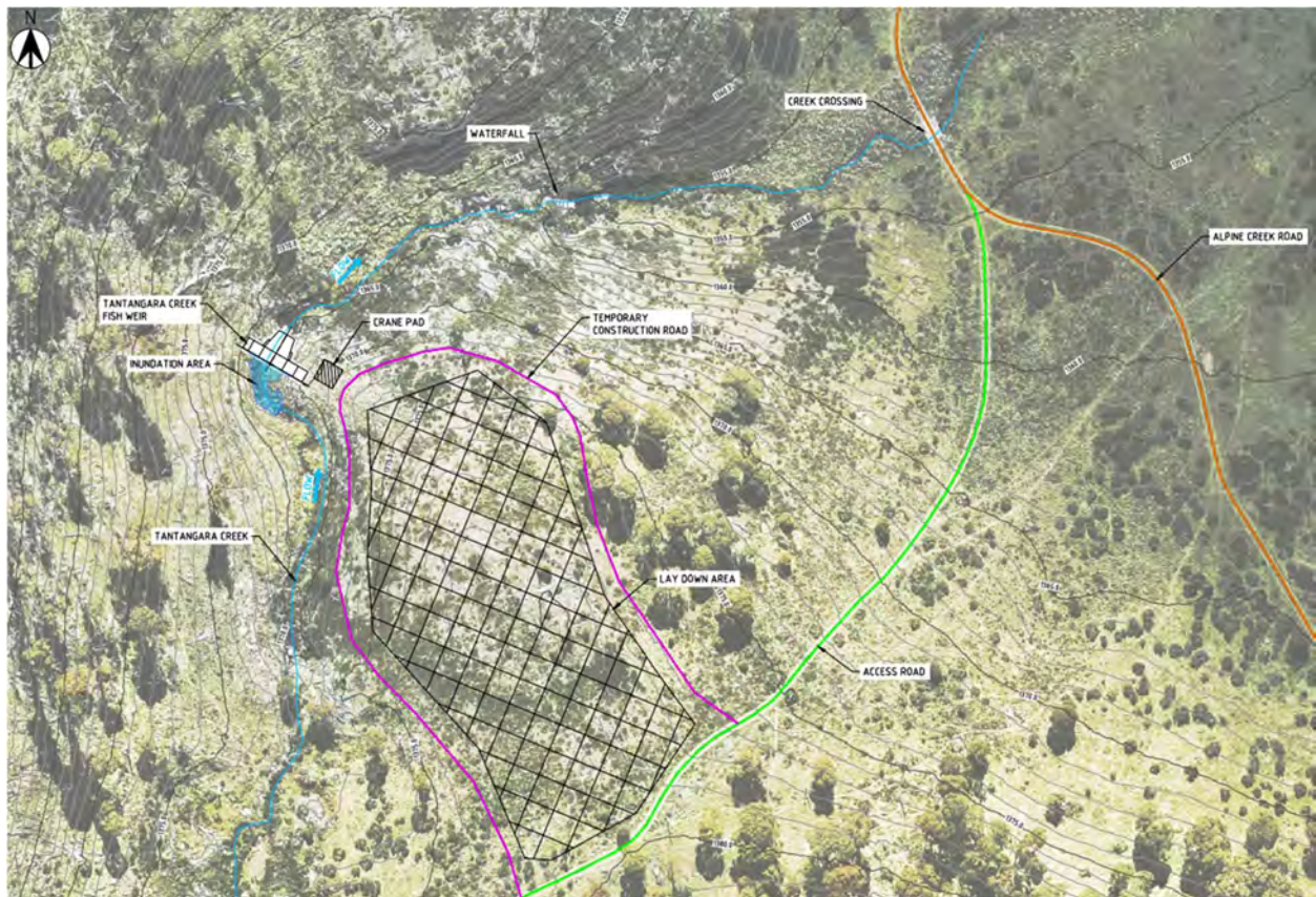
Figure 15: Concept Plan of Site Layout
