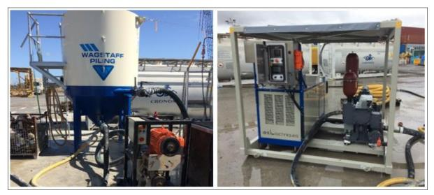
Figure 7-4 Sodium silicate system / Cement-Bentonite Slurry blending/recirculation and plunger pump (same system for both mixes)
