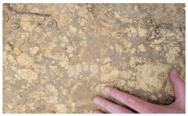
Figure 3-6 Brecciated ground on track adjacent to sink hole.
