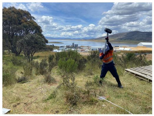
Figure 4 Seismic data acquisition (SRT Line 01)
