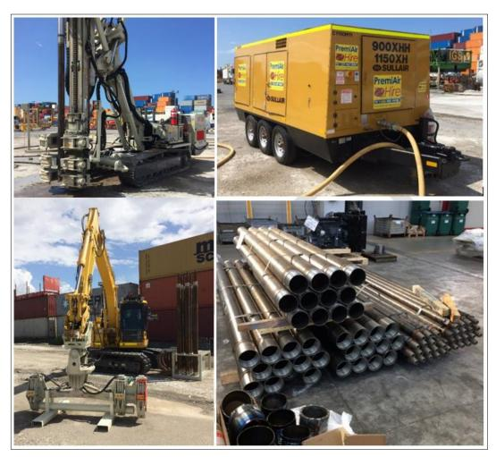
Figure 7-3 Drill rig and compressor, rod handler and rods
