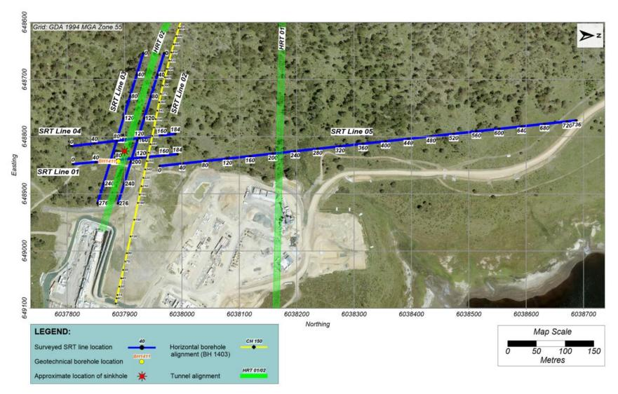
Figure 3-8 Seismic Refraction Tomography Alignment
