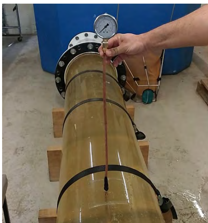
Figure 13. Calibration of the shear chamber using a total tube with a pressure gauge attached. Calibration was conducted to determine the flow velocity within the jet in front of the nozzle in the chamber and provide for the calculation of the shear strain rates to which fish were exposed.
