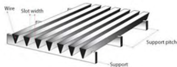
Figure 2 Wedge-wire panel (Progress Industry Group 2018).
