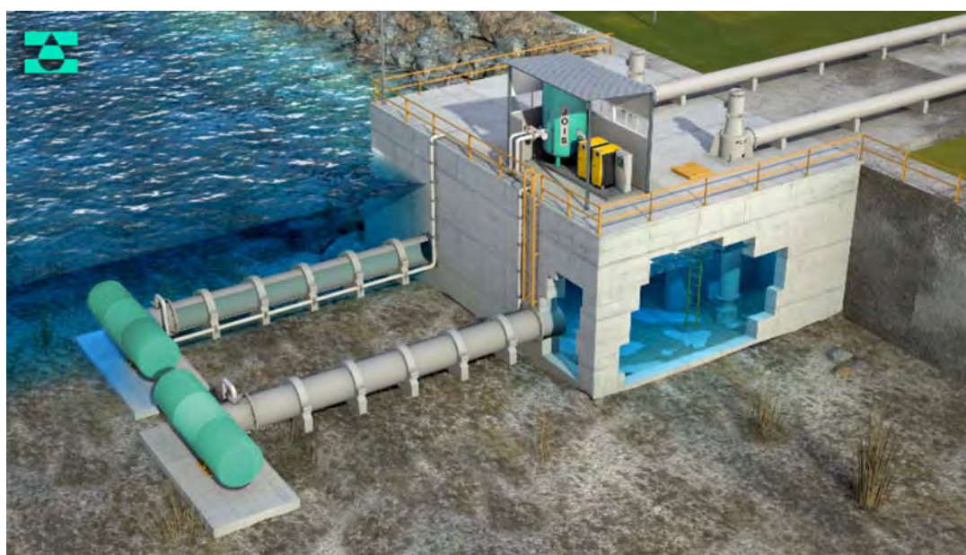
Figure 5 Visualisation of a PWWC screened intake (Aqseptence Group 2018).
