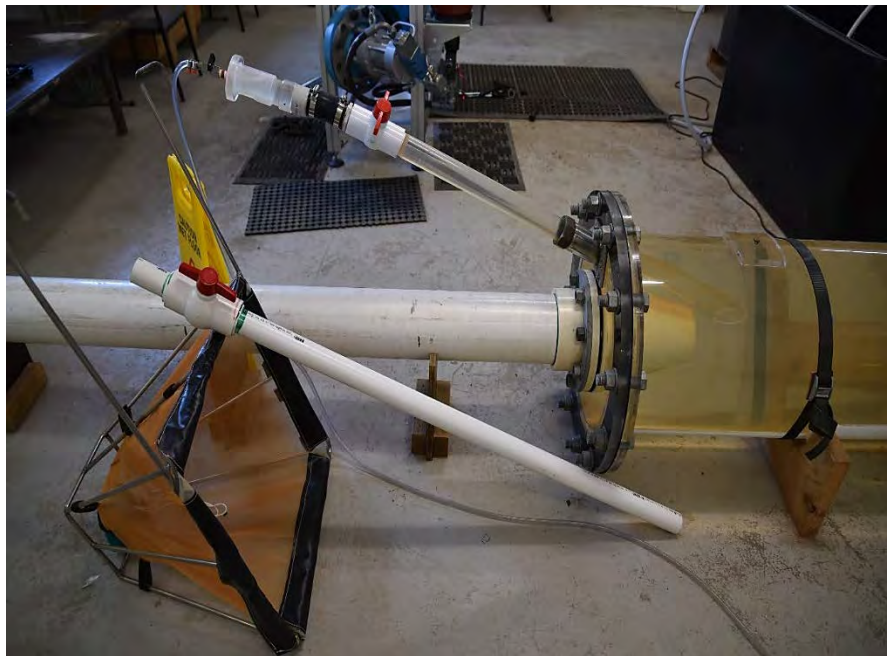
Figure 14. Deployment tube attached to the shear chamber and a duplicated deployment tube used as a control that was directed into the capture net (LHS).
