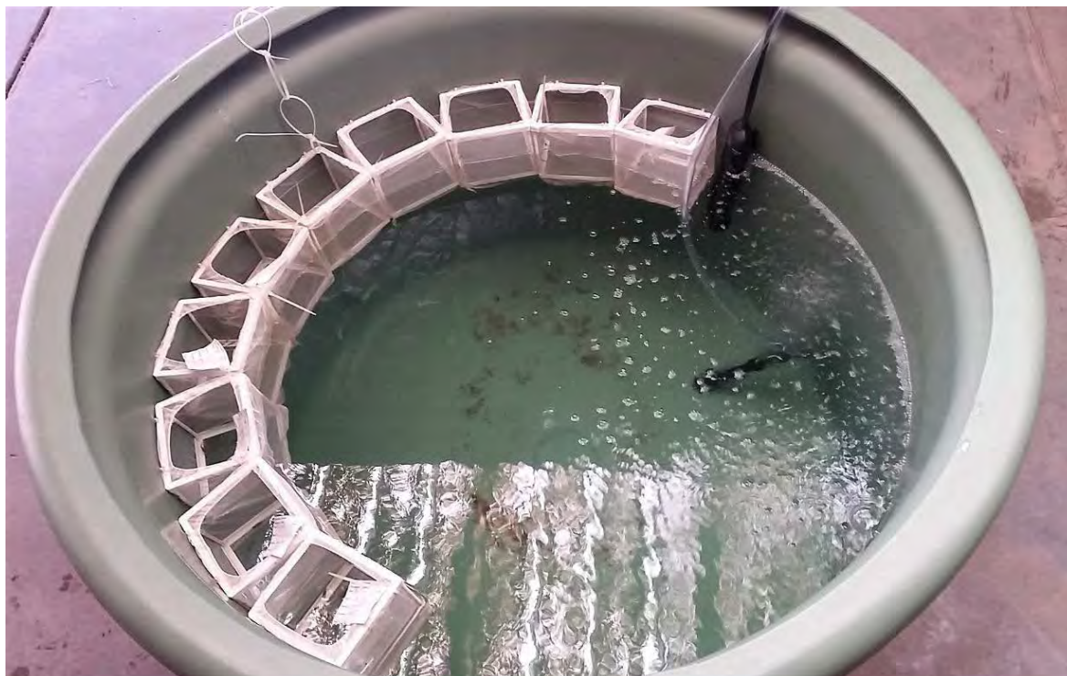
Figure 25. Holding baskets for gambusia for placement of experimental fish after pressure exposure.
