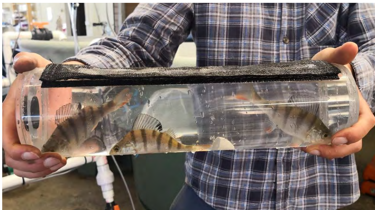
Figure 23. Photo of juvenile redfin in the Fish Pressure Chamber capsule ready to be added to the pressure chamber.
