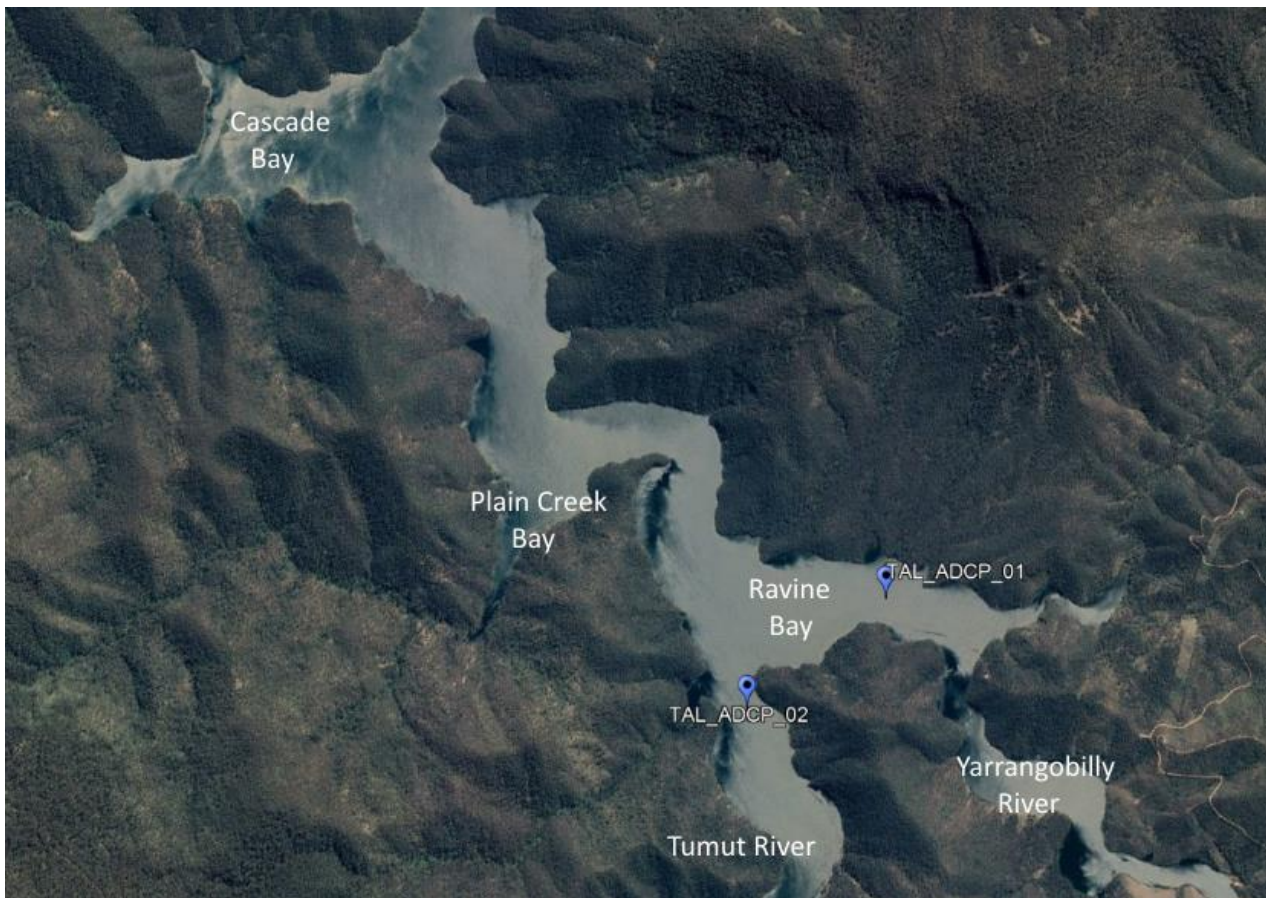
Figure D-1: ADCP Deployment Locations in Talbingo Reservoir.
