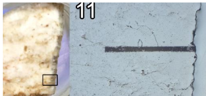
Figure 28. Sample 11 – (left) photograph of polished round with laser traverse marked with a box. (right) reflected light image of the completed 2300 µm LA-ICP-MS traverse.
