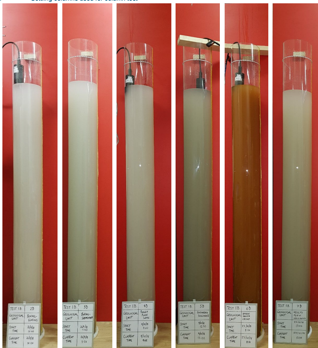
Figure 4-1 Settling columns used for column test
