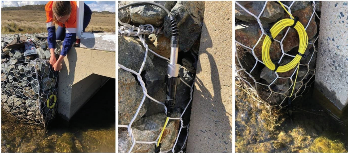
Figure 2.42 Installation of pressure logger – Eucumbene River at the culvert on the Gooandra Trail (Site 11)
