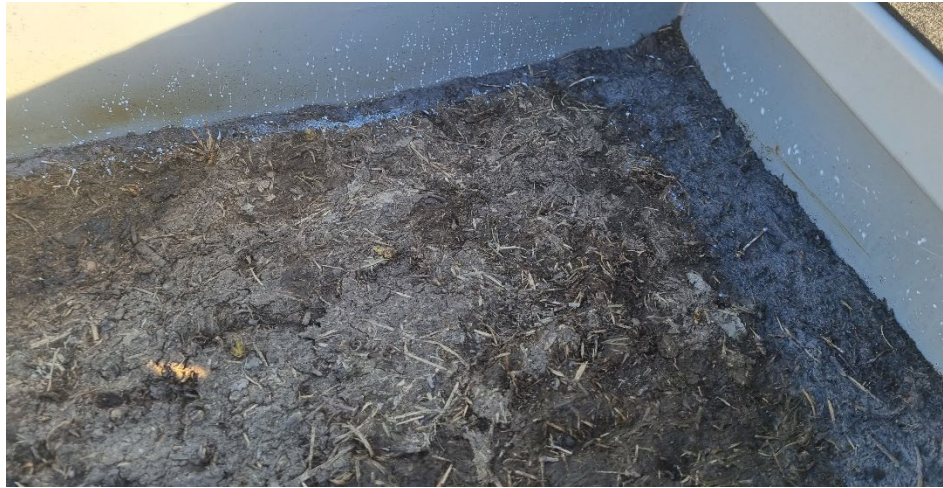
Figure 14: Stabiliser applied to the disturbed edges of the plot prior to application of overland flow.
