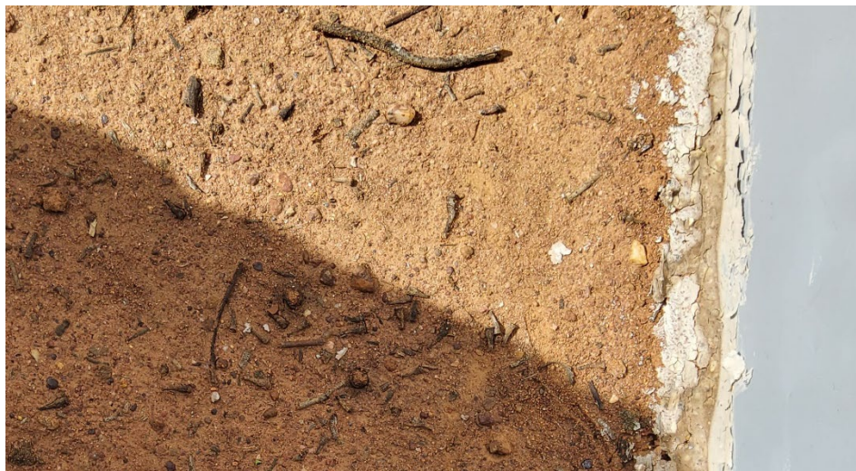
Figure 15: Bentonite (grey material) applied to the plot edge.
