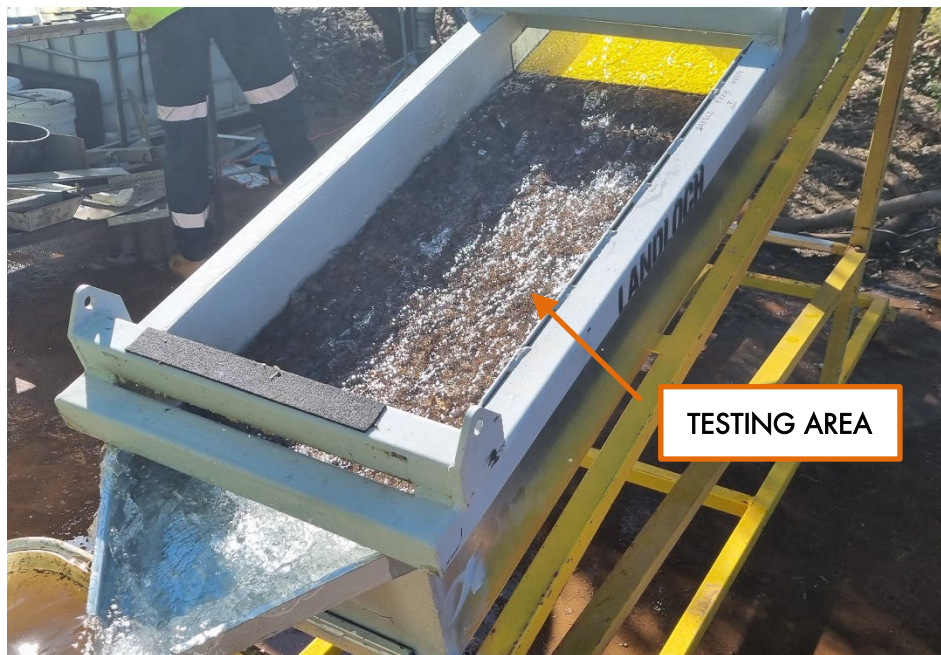
Figure 1: Hydraulic flume showing overland flowing being applied to the testing area.
