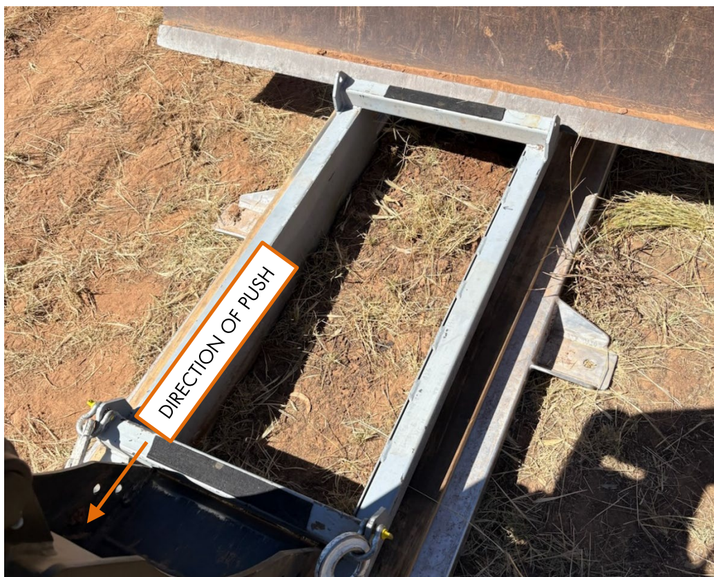
Figure 8: Sampling frame being pushed through the soil using the excavator blade.
