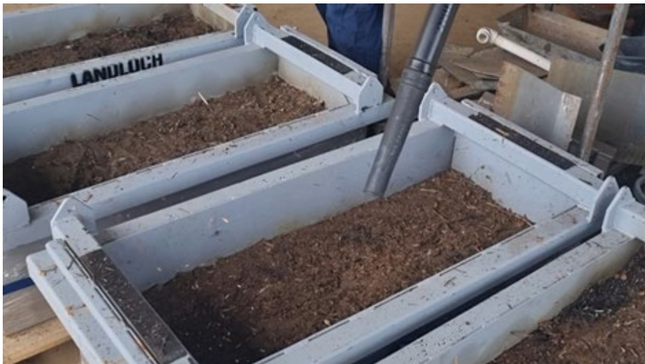
Figure 13: Removing excess vegetation debris using a leaf blower.
