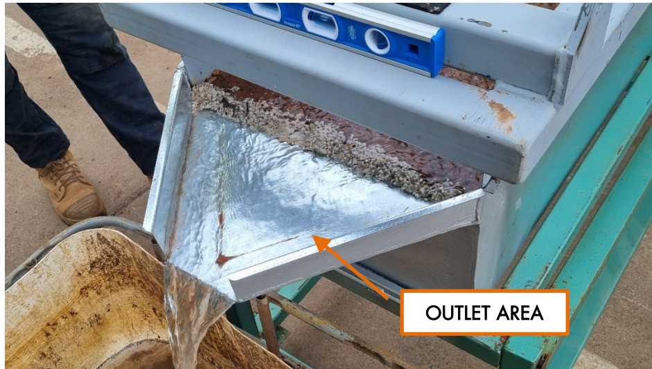
Figure 3: Outlet area shaped to allow for easier collection of samples.
