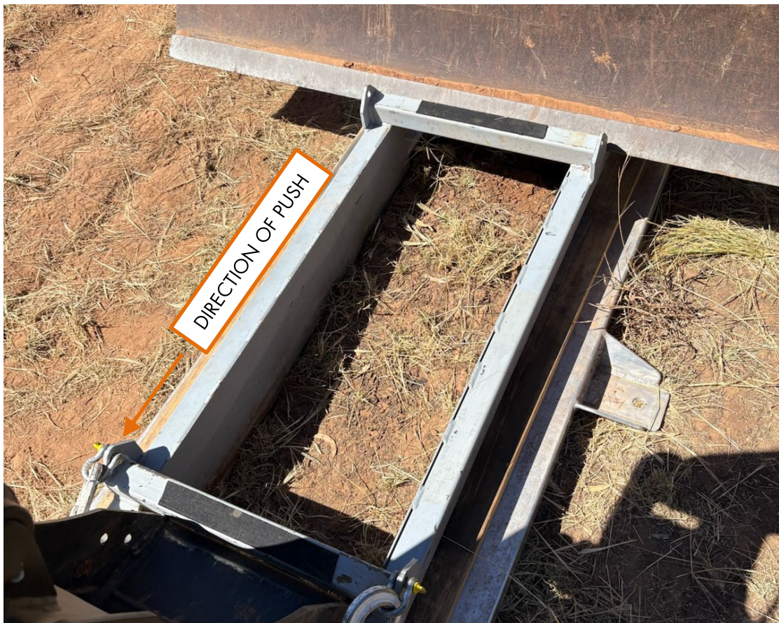
Figure 6: Sampling frame being pushed through the soil using the excavator blade.
