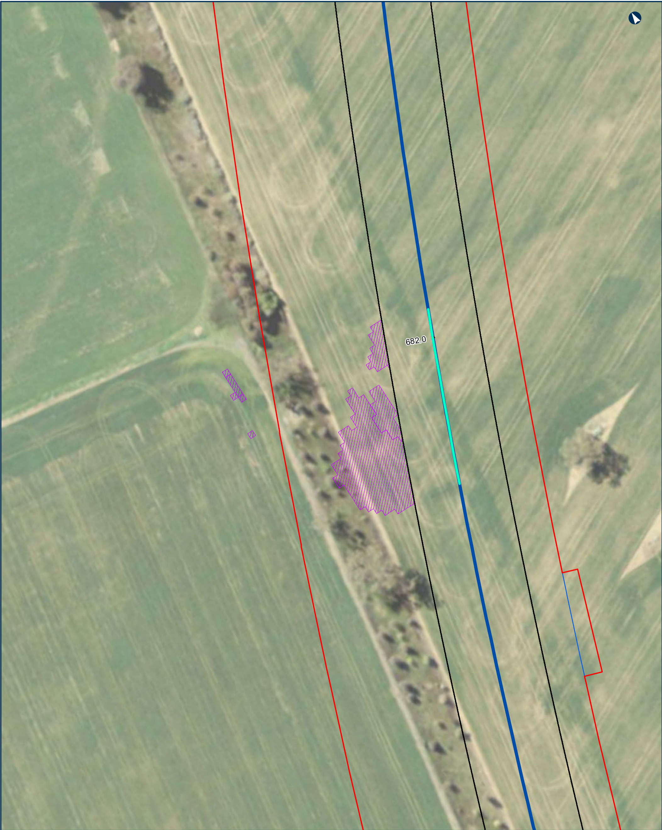
NARROMINE TO NARRABRI Residual QDL departures - 1% AEP with blockage – Reference Design Scenario Figure C2
