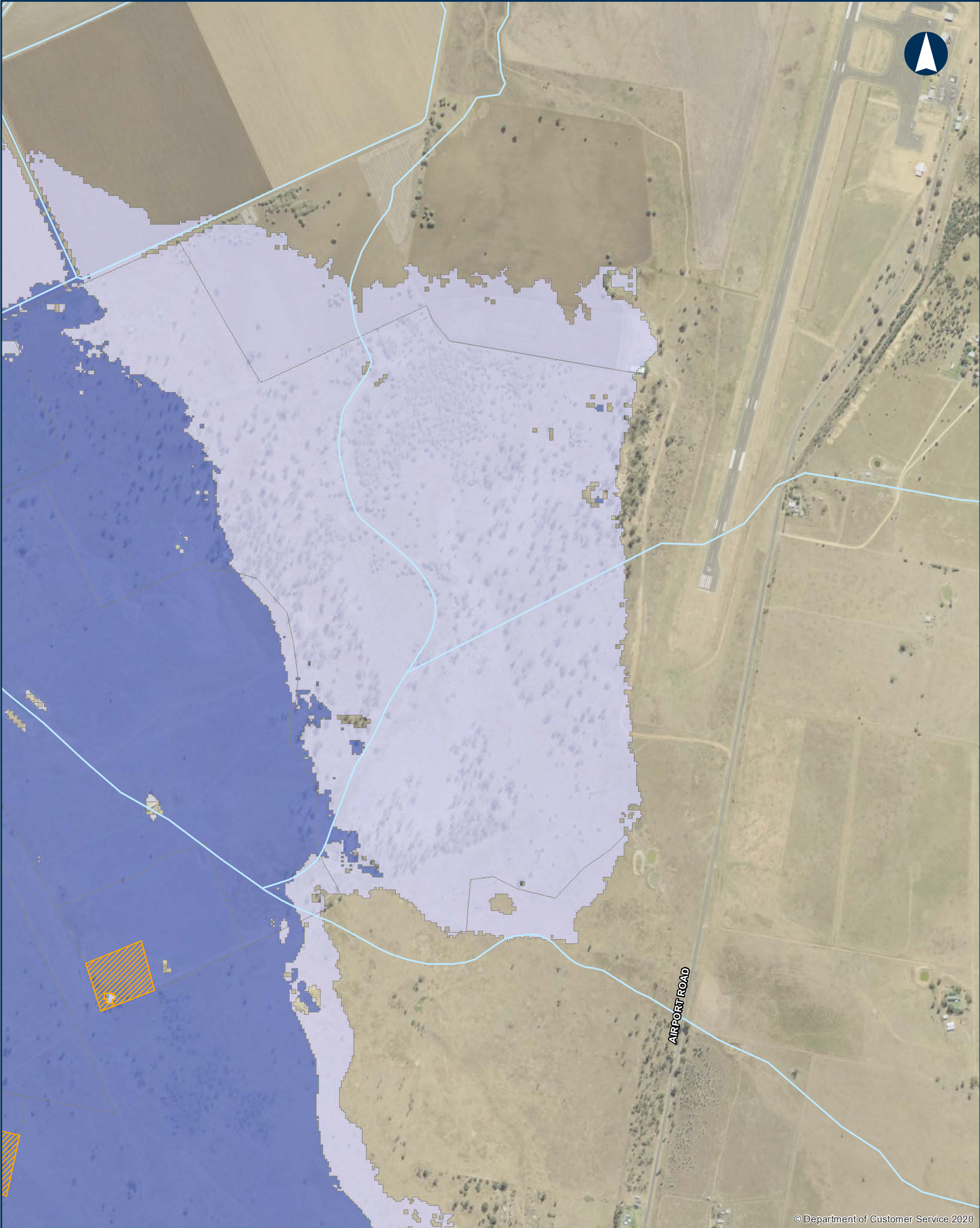
NARROMINE TO NARRABRI QDL departures - Hazard - 1% AEP with blockage - Narrabri Regional Appendix B - Figure 3.8.8
