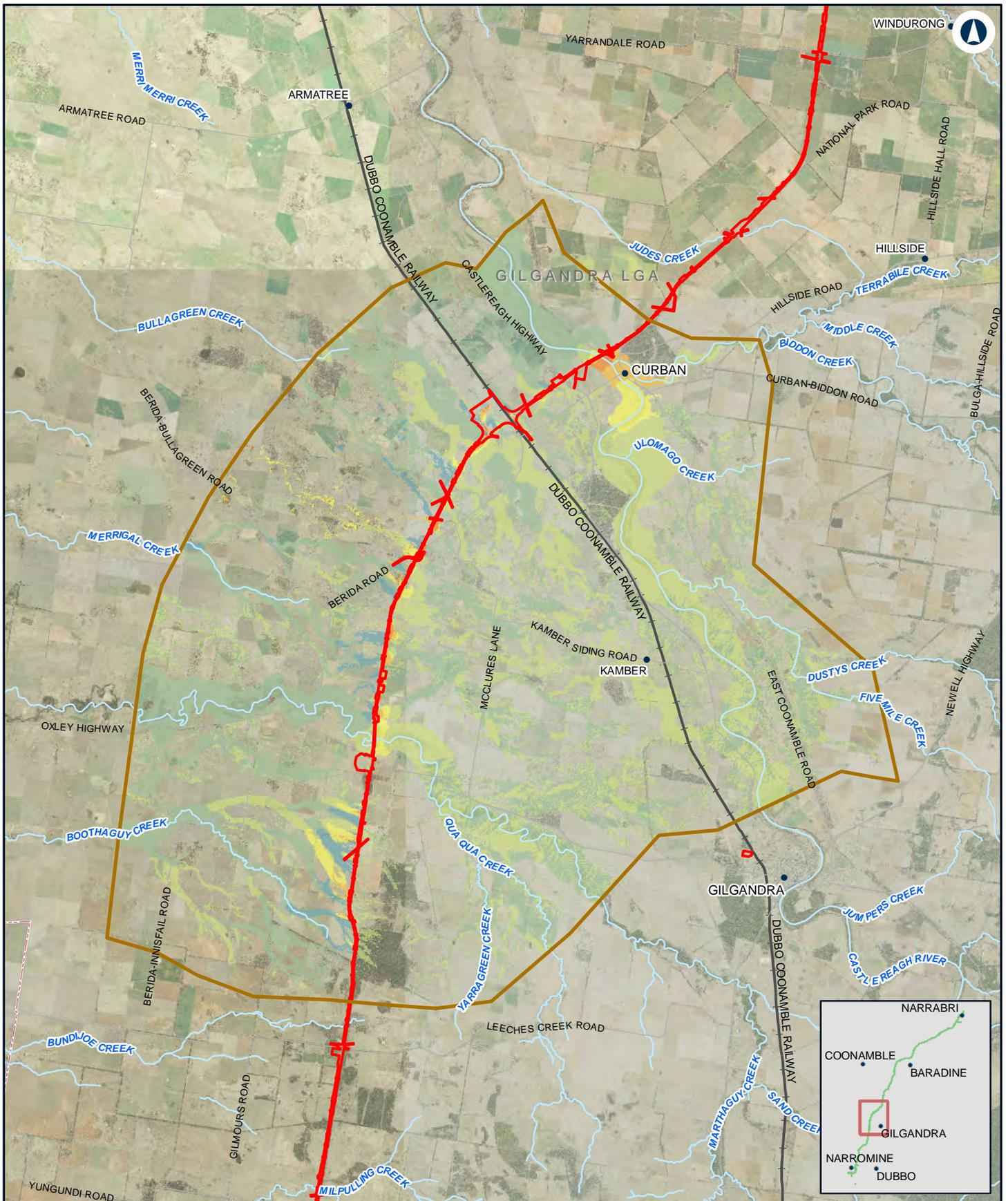
**NARROMINE TO NARRABRI** Change in peak flood level (afflux) - 1% AEP with climate change - N2N11N12Appendix G - Figure 1.5d
