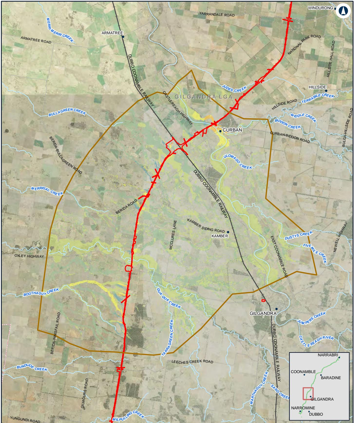
**NARROMINE TO NARRABRI** Change in peak flood level (afflux) - 2% AEP - N2N11N12
