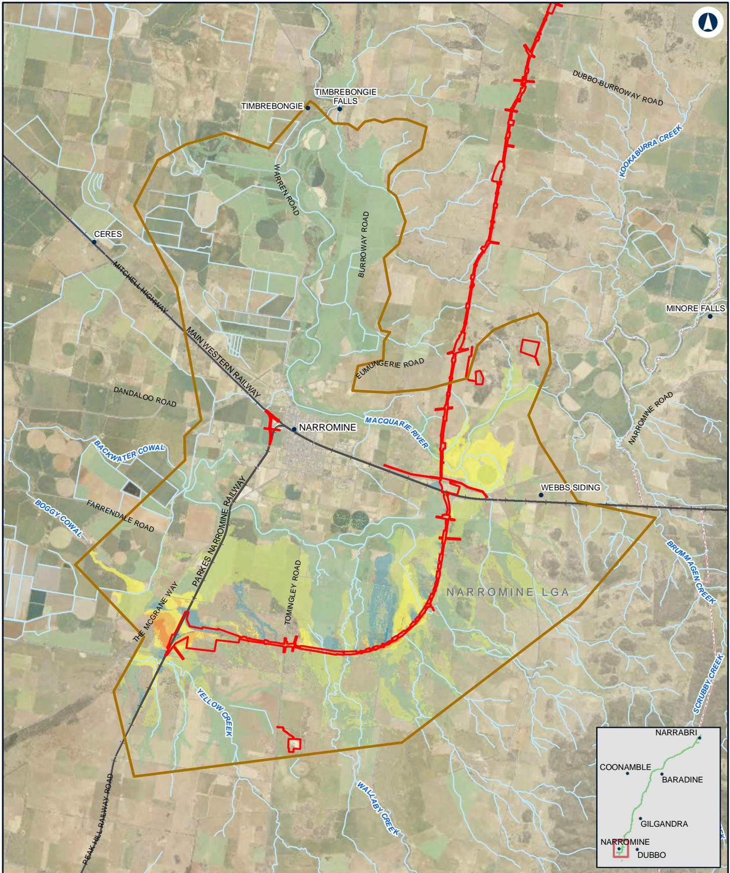
**NARROMINE TO NARRABRI** Change in peak flood level (afflux) - 2% AEP - NFM
