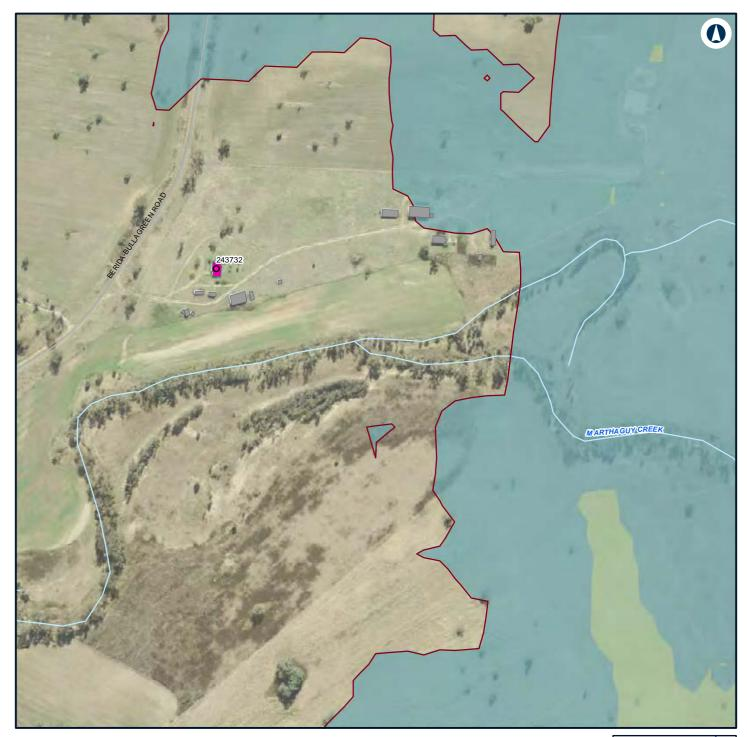
Construction noise contours, Scenario RAIL03 - Stripping Topsoil
