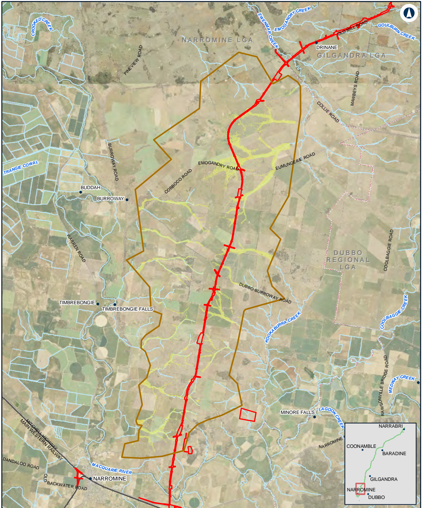
NARROMINE TO NARRABRI Change in duration - 1% AEP with climate change - N2N14 Appendix G - Figure 3.5b
