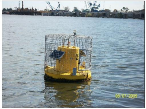
Photograph 1. Water Quality Monitoring Buoy 04
