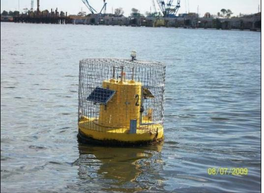
Photograph 2. Water Quality Monitoring Buoy
