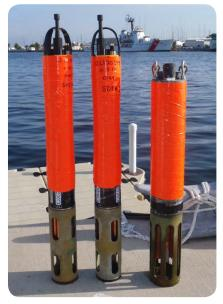
**Note:** When wrapping sondes that are equipped with depth sensors on the side, make sure that you cut small holes in the plastic wrap/ tape layers over the depth ports so that water can flow freely into the ports for correct pressure measurements.
