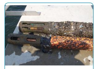
To illustrate this effect, a YSI 6600 sonde was deployed without any kind of anti-fouling protection. Alongside it, an EXO2 sonde wrapped in plastic wrap and covered in high-visibility Duck® brand duct tape was deployed.
