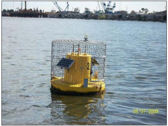
Photograph 1. Water Quality Monitoring Buoy 04
