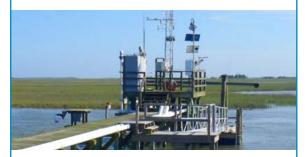
At a long-term monitoring station in a productive South Carolina estuary, a YSI EXO2 sonde and YSI 6600 sonde with anti-fouling components were deployed. The sondes were connected to a data logger that transmitted real-time data back to our office.
