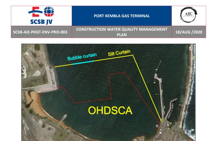
Figure 6 Approximate Silt and Bubble Curtain alignment in Outer Harbour
