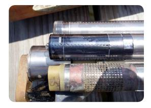
**Sensor Guards:** You can also prevent debris and small animals from entering the sensor guard by using 0.25-inch plastic mesh around guard. Wrap the mesh around the outside of the guard 1.25 times and secure with a cable tie or rubber band. The mesh can also be sprayed with copper-based anti-fouling paint (see tip 10 below).
