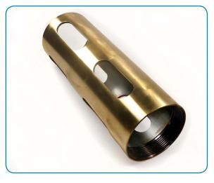
*Copper-alloy sensor guards effectively deter biofouling settlement on sensitive water quality sensors. As the guard ages, it naturally gains a patina.*
