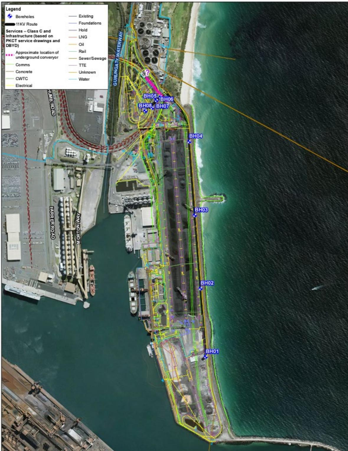
Figure 6.3 Site layout showing borehole locations
